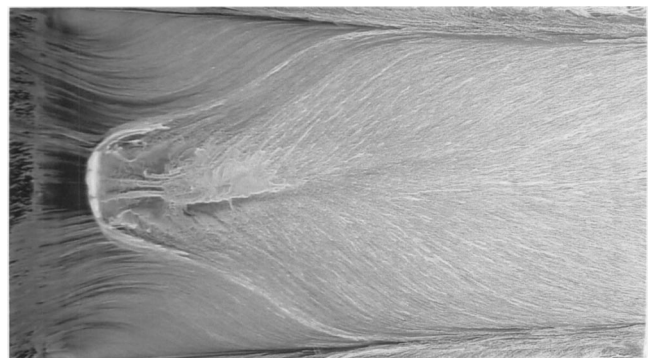
Fig. 10 Surface flow visualization on the ramp: 20 deg diffuser, h_r / (d \times \theta) = 0.694 , 30 m/s. Flow from left to right. Picture area corresponds to the ramp area.
